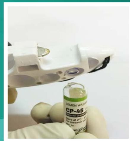
Figure 5c: Show the recommended ampoule opener (Arian Biotech System) to avoid sharp injuries & media spillage
