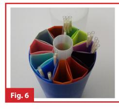
FIG 6. Goblet with visotubes and 0.5 ml sperm straws. Different colours help in easy identification of the sample. CBS High Security straws are placed in goblets for storage in freezers. Goblets come in 8 different colors and their sub-compartments (called visotubes) in 12 different colors. In the Daisy configuration, goblets hold 12 visotubes of different colors and can hold a maximum of 168 CBS straws of 0.3 ml or 0.5 mL
