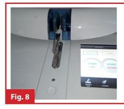
**FIG 8. SYMS III** sealer for high security straws (manufactured by Cryobiosystem). The **SYMS III** thermally seals 0.3 mL, 0.5 mL and 2 mL CBS<sup>™</sup> High Security straws as well as CBS<sup>™</sup> High Security Vitrification straws and CBS<sup>™</sup> High Security Tubes for top quality cryopreservation of biological samples. A color touch screen that can be used while wearing laboratory gloves is present.
