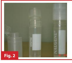
FIG 2. Cryovials from different manufacturers vary in size and placement of cap rings. Cryocell vials have an external gutter for  $LN_2$ . NUNC cryovials have an internal threading's. These are mounted on the aluminum vial holders by plugging mechanism.
