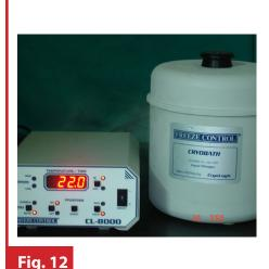
**FIG 12. Computer-controlled freezer:** (Freeze Control temperature controller, cryochamber and cryobath)
