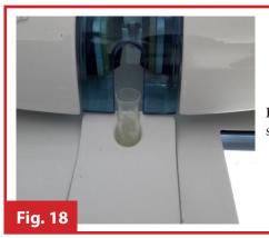
FIG 18. If we are using CBS cryostraws ,we have to Load the cryovial on SYMS III sealer.
