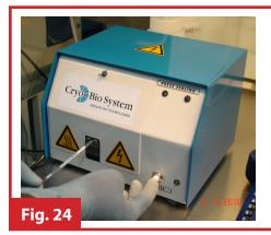
**FIG 24.** Filled and labeled straws are heat sealed using a heat sealer. This makes the packaging relatively aseptic.
