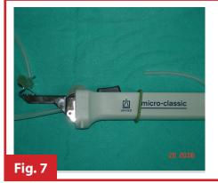
**FIG 7. Micro-aspirator** (manufactured by Cryobiosystem) used to manually fill sperm straws. The micro-aspirator is used to manually fill straws without any risk of contamination.
