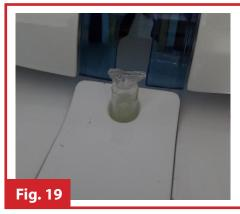
**FIG 19.** Sealing of cryotube using SYMS III sealer has been done and the cryotube is hermitically sealed.
