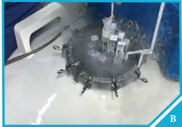
Fig.8b: Proper labelling of the aluminium cryocanes for easier identification of the location of carrier devices.
