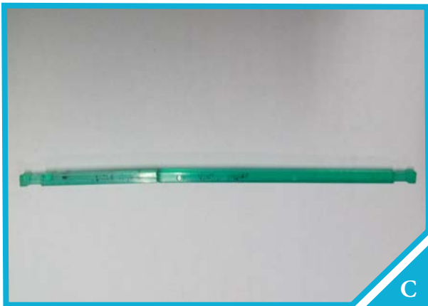
Fig.8c: If the devices are not marked properly or marked with sub quality pens the writing comes off and it is difficult to identify the device later at the time of warming.
