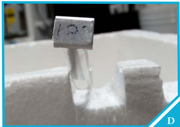
Fig.8d: If the aluminium Cryocanes are not marked properly or marked with sub quality pens the writing comes off and it is difficult to identify the device later at the time of warming.
